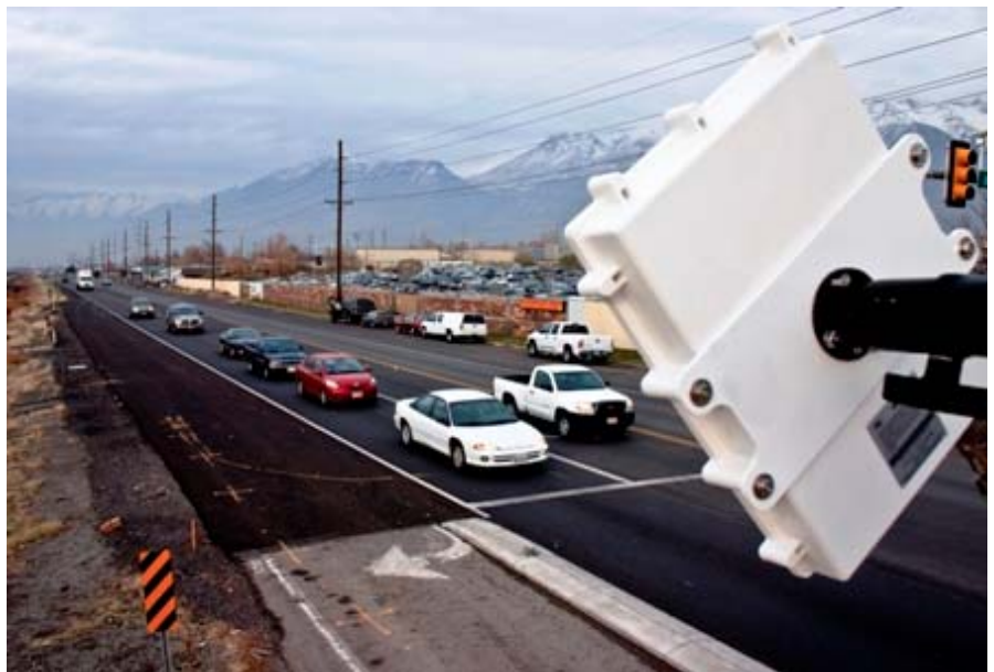
SmartSensor Advance mounted at an intersection
