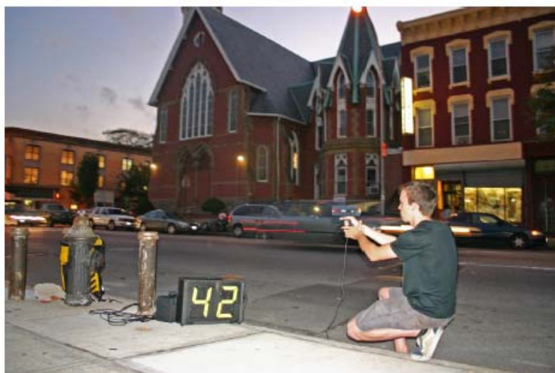
A Transportation Alternatives researcher measuring vehicle speeds in New York City.
